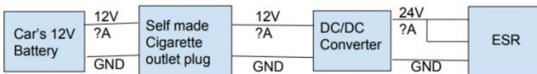
For the Lidar, we were not able to get to powering it, but since it also uses a 24V DC power similar to the ESR radar, we plan on using a similar method and extending the power applied to the ESR to also power the Lidar. We have tested getting information from it and feeding it through ROS. We are able to get the information and manipulate it now for the controls tea.
