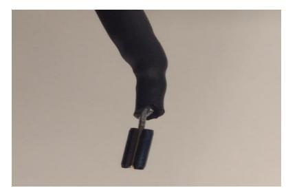
After soldering the metal rod clamp onto the tip of the wire, we assembled the contact to the connector. The connector would then have a firm contact with the wire which now enables us to gather more accurate output data rather than simply struggling to get the node connections in our previous experiments.
