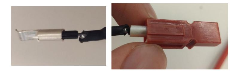
With the wires made, we can look forward to running more tests and getting use to the configurations. We made a total of eight testing wires for the 4 pair of nodes that are available on the RigRunner.
