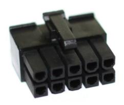
The PX2 will use a 10 pin PCI-E port which was mentioned in the previous log(Although the PX2. The wire connecting to the RIg Runner will be configured with a 12V output which is the power needed for the PX2. Since this is a VGA power supply cord, we will need a way to adapt it to a single wire that can be then converted to the RigRunner port. The prototype adapter involves the following parts:
